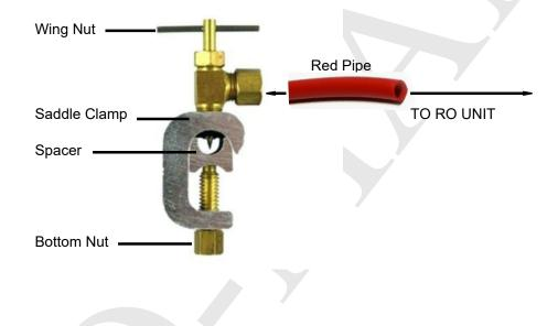
• Now fit the saddle valve to the 9 or 15mm copper cold water supply pipe ensuring that the spacer is fitted closely to the pipe, then tighten the lower bolt with a spanner. You can now connect the red ¼" pipe, which will feed the RO system, by simply pushing it into the saddle valve as far as it will go and then gently pulling back to ensure that it is gripped securely.
